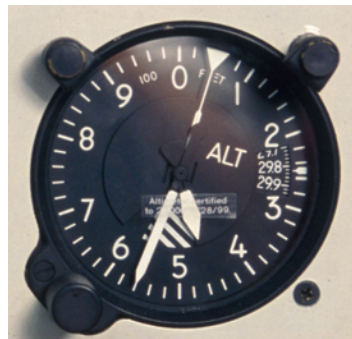
Name: altimeter Altitude: 4 , 560 feet
