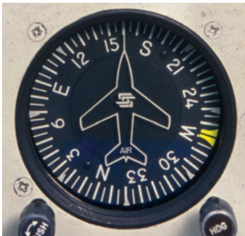
Name: heading indicator Heading: 160 degrees
