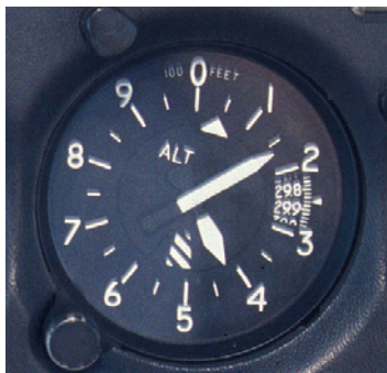
Name: altimeter Altitude: 4 , 160 feet
