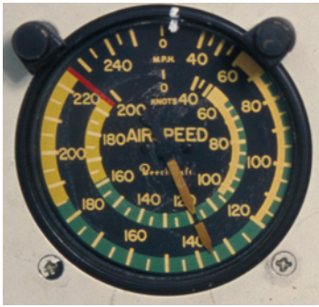
Name: airspeed indicator Speed: 120 knots 135 mph
