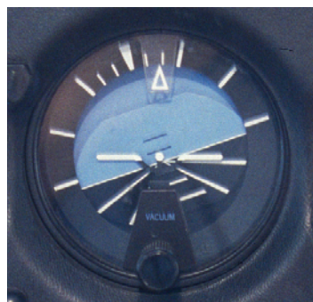
Name: attitude indicator Plane is turning: ✓ Right? Left?
