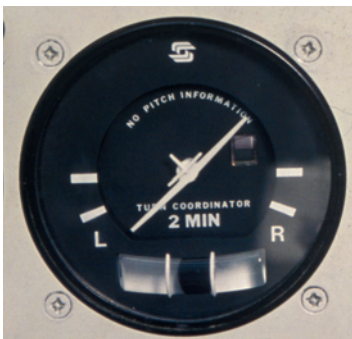
Name: turn coordinator Plane is turning: Right? ✓ Left?
