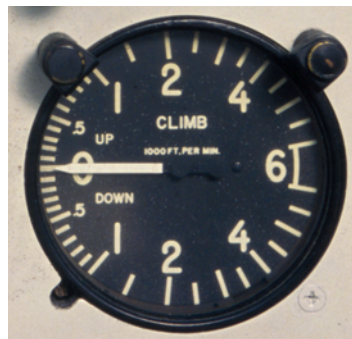
Name: vertical speed indicator Is plane climbing? Flying level? ✓ Descending?
